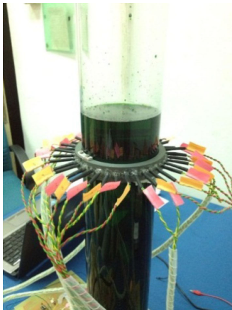
Fig. 6 The sample of water contaminated by 35 ml of food colouring
