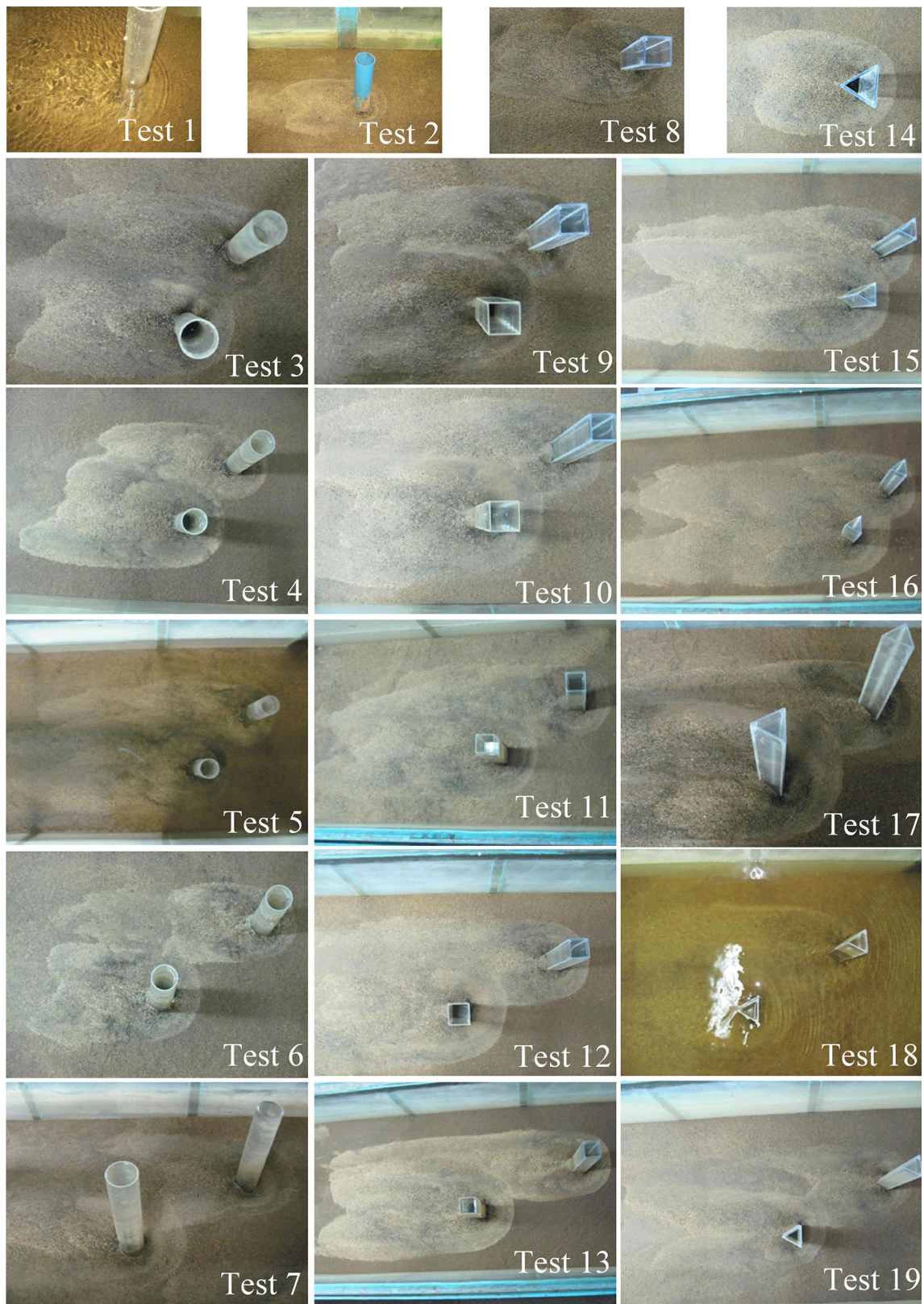
Fig. 2 Scour-affected zones around circular, square and triangular piers for tests 1–19
