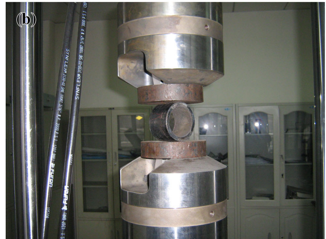
Fig. 2 Schematic diagram (a) and photograph (b) of the compression test
