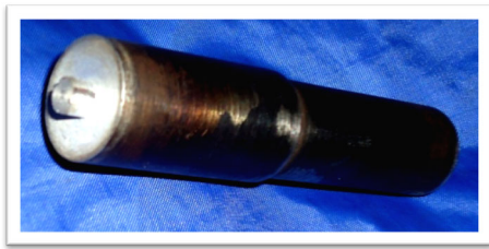
Fig. 1 Concave shoulder FSP tool with straight flutes
