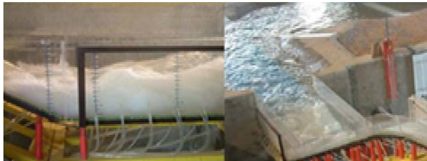
Fig. 2 Flow formation inside the stilling basin with the discharge of 300 (m 3 /s) [20,21]
