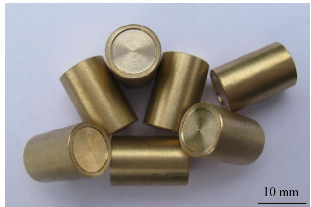
Fig. 2 Typical appearance of the specimens of the lead-free machinable brass before the hot compression tests
