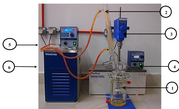
Fig. 2 Experimental set-up used to perform biodiesel production. (1) 1L Jacketed glass batch reactor (Brand: Favorit); (2) reflux condenser; (3) overhead mechanical stirrer (IKA EUROSTAR digital); (4) circulating water bath; (5) hoses; (6) Refrigerator
