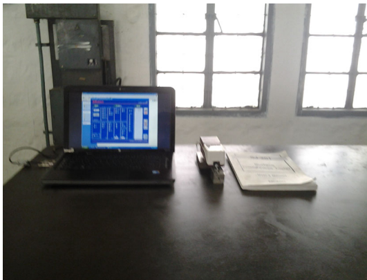
Fig. 3 Surface roughness measurement set-up 2 with Mitutoya SJ-201 surf tester
