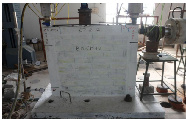
Fig. 4 2% HFRC frame specimen—load set-up
