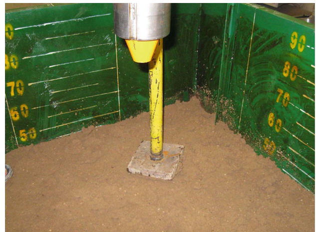
Fig. 6 Compaction procedure using special tamper
