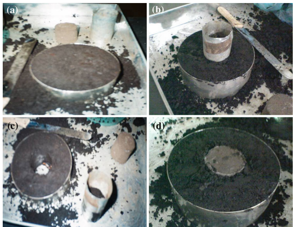
Fig. 3 Column installation procedure: a Undisturbed peat sample. b Thin-walled metal tube cutters inserted in the undisturbed peat. c Sample with hole prepared for the column. d Stabilized peat column inserted in the undisturbed peat sample
