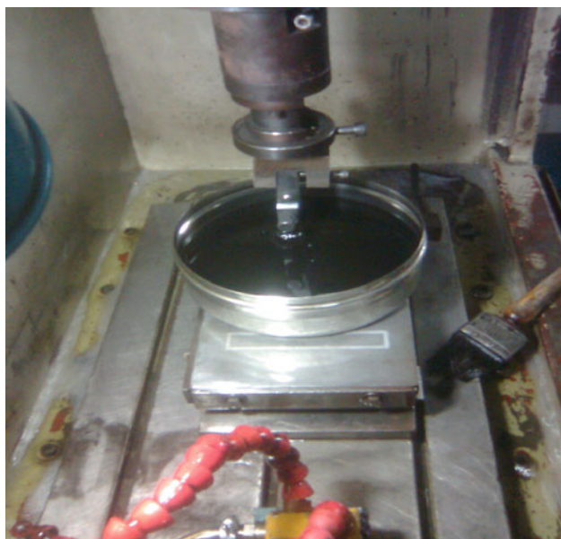
Fig. 4 EDM set up using SWCNT
