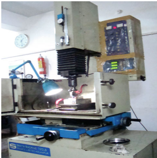
Fig. 3 Electric discharge machining (SD35-5030)
