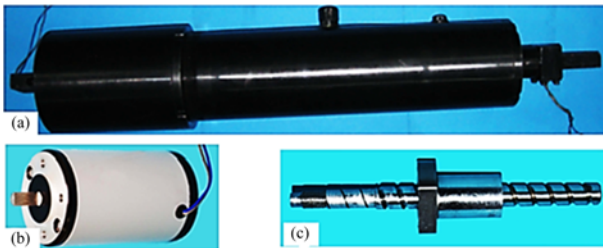
Fig. 66. (Color online) Photographs of the proposed MRD. (a) MRD, (b) the generator, and (c) the ball screw (Xinchun et al. , 2015).
