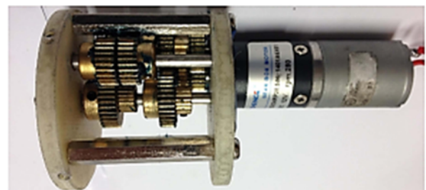
Fig. 64. (Color online) Image of motion rectifier prototype mounted with ZGA 25RP motor (Chu et al. , 2016).
