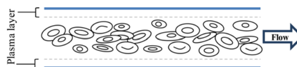
Fig. 3. (Color online) Sketch of the formation of a plasma enriched layer near the vessel walls and accumulation of RBC at the center of the vessel when blood is flowing (wall effect).
