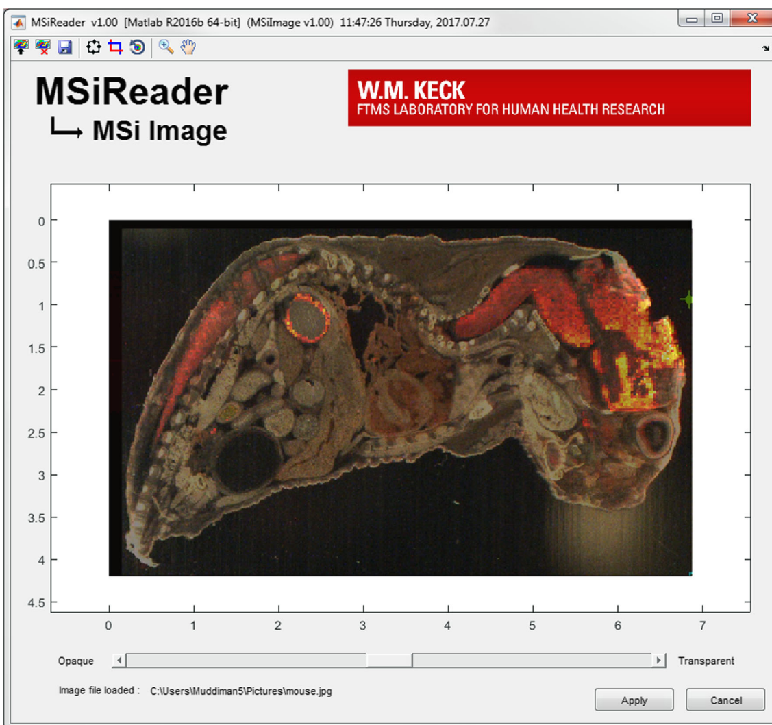
Figure 4. MSiImage tool for overlaying an optical image with the ion image of putatively assigned desmosterol ( m/z 367.3363, [M+H^+-H_2O]^+ ) obtained in a whole-body IR-MALDESI analysis 2-d-old neonatal mouse
