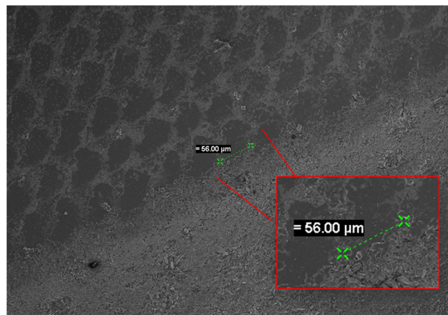
Figure 3. SEM image of an ablation pattern demonstrating an external spot diameter of 56 \mu\text{m} and an internal diameter of 50 \mu\text{m} representing an 83% ablation efficiency of the laser. The single shot laser ablation shape can be seen in Appendix 1
