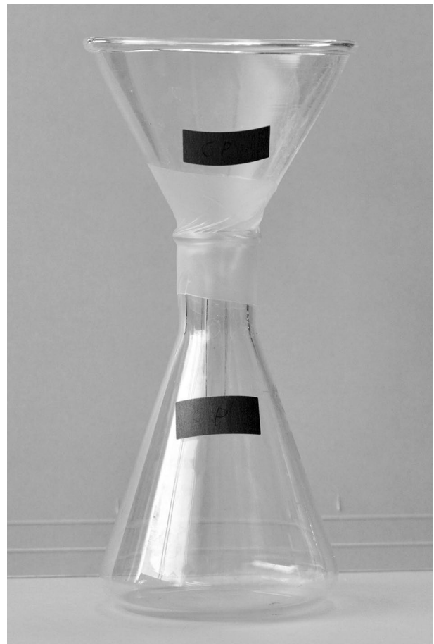
Fig. 1 A simple trap devised to conduct a bioassay of the male response of Bactrocera correcta to \beta -caryophyllene (CP) or methyl eugenol (ME)
