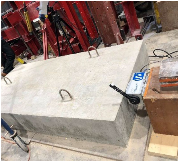
Fig. 3 Scalable automatic modal (SAM) hammer by Wavehit®
