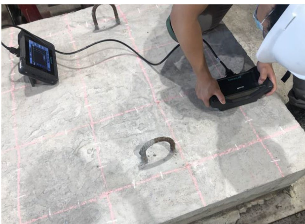
Fig. 11 Ultrasonic shear-wave tomography measurement on a grid of 10 by 22 points with the grid size as 100 mm using PUNDIT PL200
