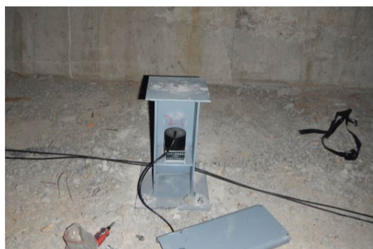
(a) Acceleration sensor
