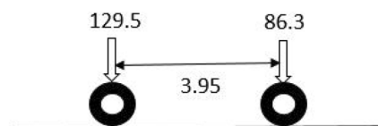
(a) Axial load distribution for 22T vehicle
