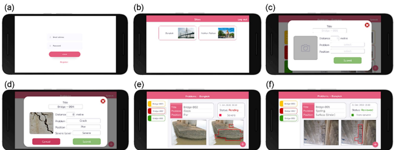
Fig. 10 Complete inspection system user interface. a login page, b main menu page, c image acquisition and defect information page, d acquired bridge substructure image and defect information with
