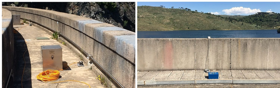
Fig. 2 On the left: centralized acquisition system with cables; on the right: portable recorder with GPS antenna
