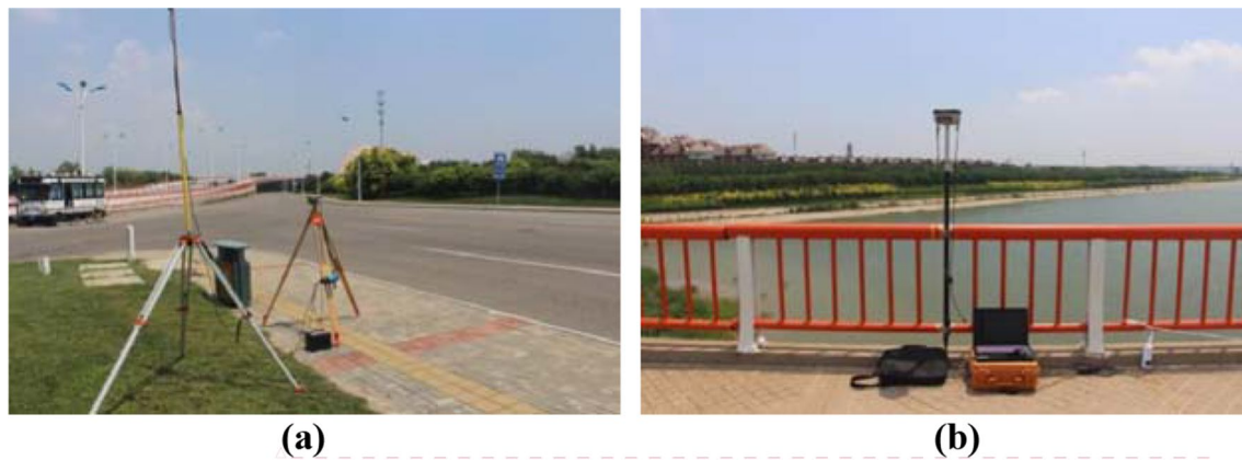
Fig. 9 a The arrangement of GNSS reference station; and b the arrangement of GNSS rover stations
