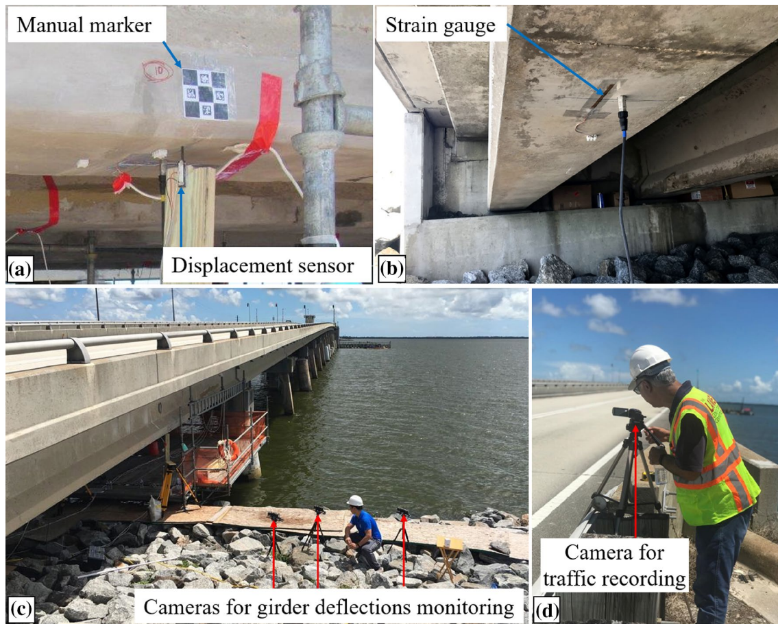
Fig. 9 Sensors and camera instrumentation details for the experiment
