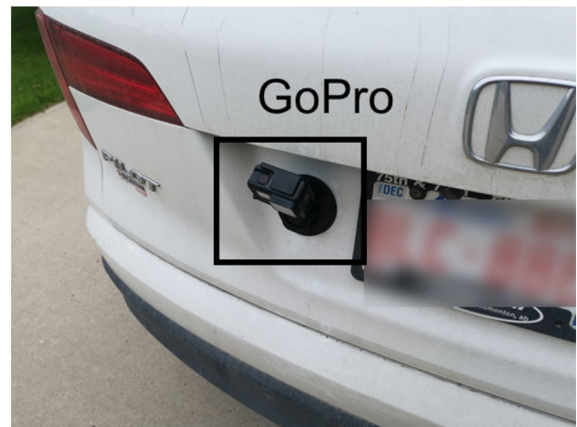
Fig. 13 Mounting of GoPro sport camera
