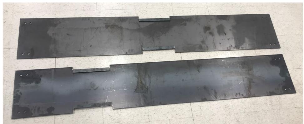
Fig. 6 Local damage created by section area reduction
