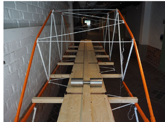
(b) Rolling mass on the bridge.
