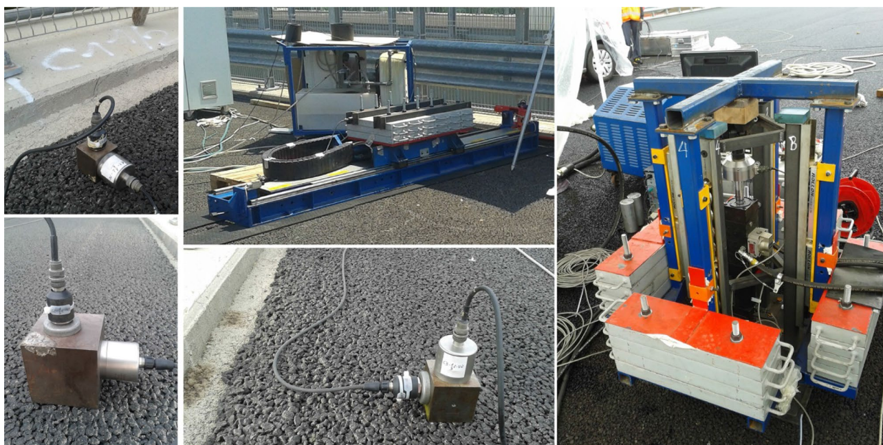
Fig. 7 Hydraulic actuator and accelerometers of the system for experimental modal analysis
