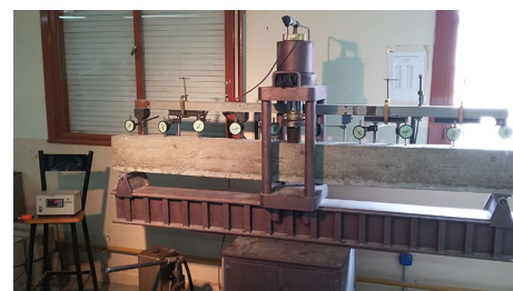
Fig. 8 View of Beam 01 when the crack was caused
