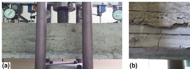
Fig. 10 Crack of Beam 01. a General view. b Detailed view
