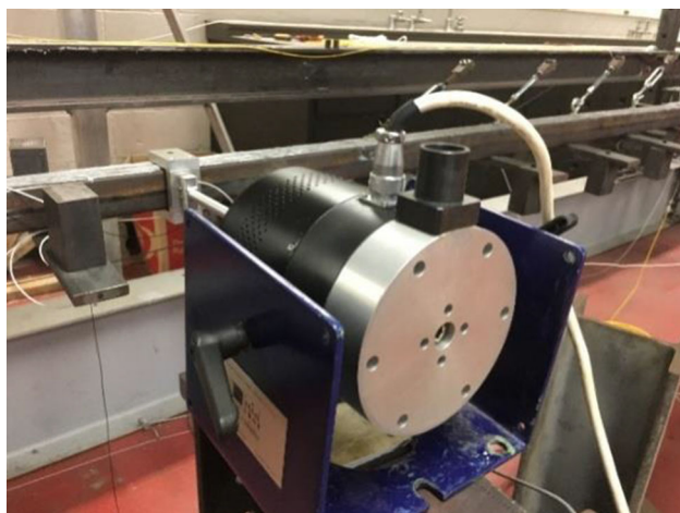
Fig. 10 Shaker connected to the bridge at mid-span
