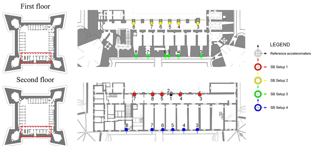
Fig. 5 Layout of the uniaxial accelerometers for the four setups (S1-red, S2-yellow, S3-green and S4-blue) used for the execution of AVT on the first (a) and second (b) floors of the monument (colour figure online)
