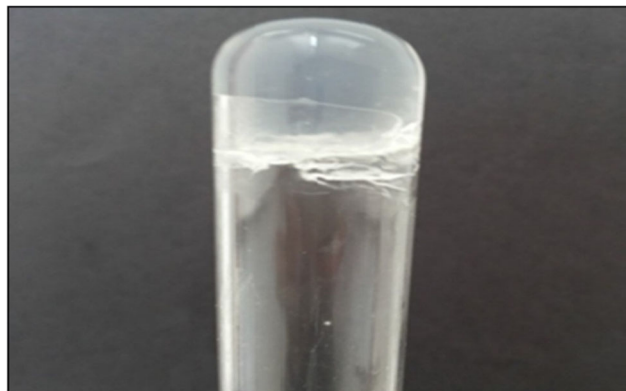
Fig. 2 Photograph showing the appearance of in situ gel formed in simulated nasal fluid
