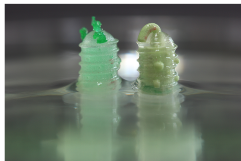
Fig. 2 Results of a preliminary experiment with super absorbent polymer in a rapid prototyped IMDDS. Only SAP inserted (left); mock drug material and SAP inserted (right)
