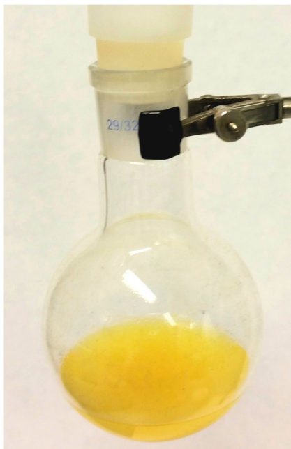
Fig. 1 Ready-to-inject dispersion (mean particle size of 2.8 \pm 0.7 \mu\text{m} ) of elacridar for i.v. infusion in nonhuman primates. The preparation was achieved using a co-solvent strategy, resulting in a final concentration of 5 \text{ g L}^{-1} elacridar with tetrahydrofuran (5% w/v) in aqueous D-glucose solution (2.5%, w/v)
