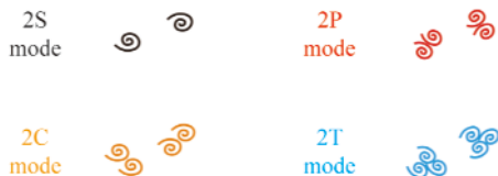
Fig. 5. Sketch of the vortex shedding modes during lock-in.
