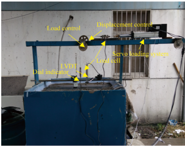
Fig. 5. Suction caisson model test.
