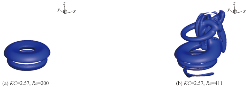
Fig. 6. Flow fields for oscillating circular disks. The vortical structures around the disks are identified by \lambda_2 criterion and the iso-surfaces of \lambda_2=-10f^2 are shown. f=1/T is the oscillating frequency.
