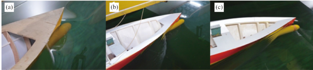
Fig. 32. Bow wave patterns of ship models with different \lambda values at Fr = 0.152 : (a)–(c) Models 1–3, respectively.
