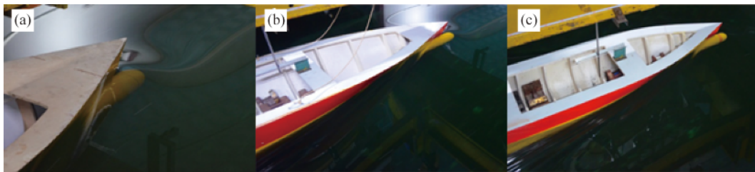
Fig. 33. Bow wave patterns of ship models with different \lambda values at Fr = 0.282 : (a)–(c) Models 1–3, respectively.
