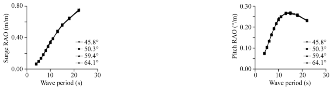
Fig. 10. Surge and pitch RAOs of the platform for different mooring fairlead slopes – intact line condition.
