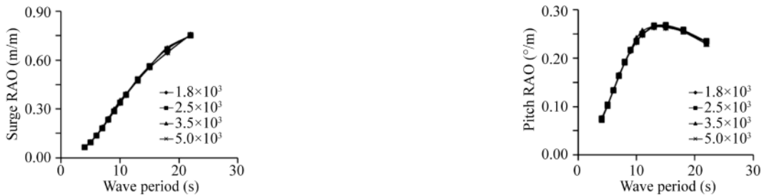
Fig. 14. Surge and pitch RAOs of the platform for different mooring pretensions – intact line condition (Line pretensions mentioned in figure are in kN).
