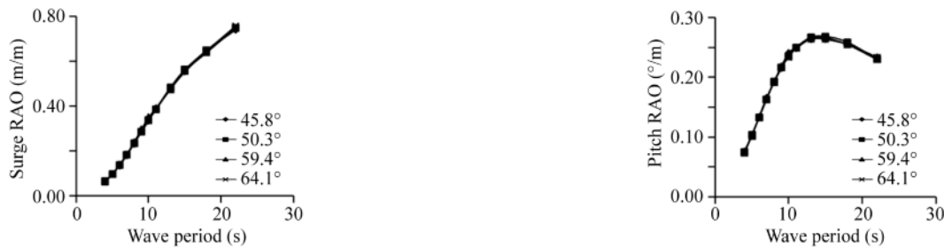
Fig. 11. Surge and pitch RAOs of the platform for different mooring fairlead slopes – damaged line condition.
