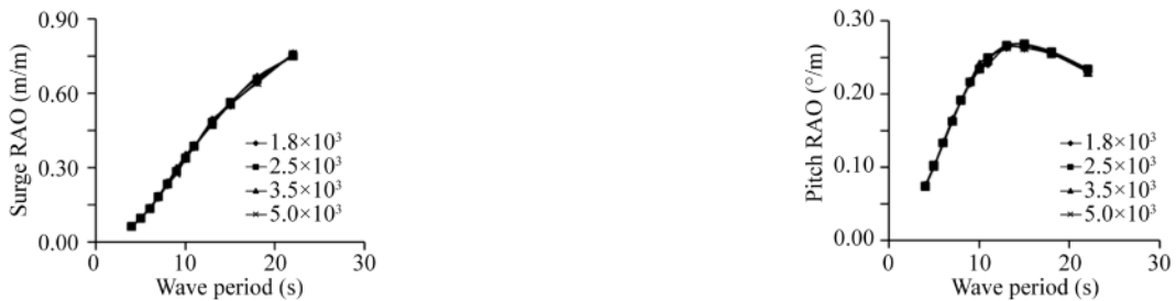
Fig. 15. Surge and pitch RAOs of the platform for different mooring pretensions – damaged line condition (Line pretensions mentioned in figure are in kN).
