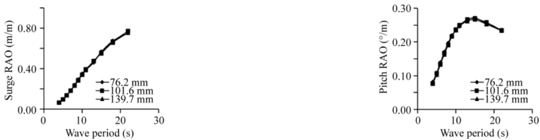
Fig. 6. Surge and pitch RAOs of the platform for different mooring diameters – intact line condition.
