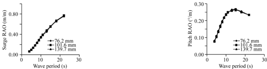
Fig. 7. Surge and pitch RAOs of the platform for different mooring diameters – damaged line condition.
