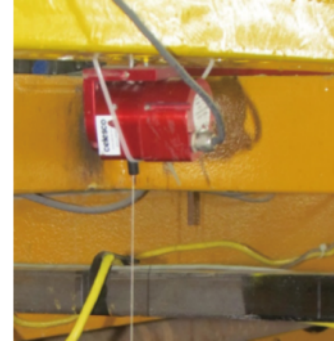
Fig. 5. Mechanical-electrical draw wire sensor being used to measure the structure motion.
