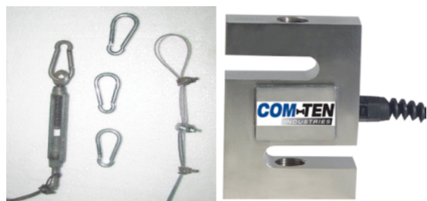
Fig. 4. Load cell and equipment being used to measure the mooring line forces.
