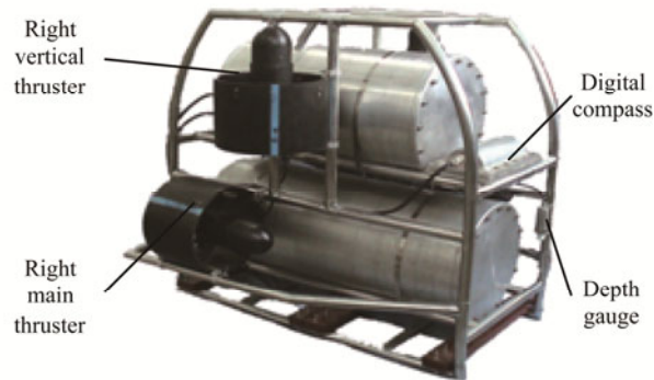
Fig. 3. “Beaver” AUV test prototype.
