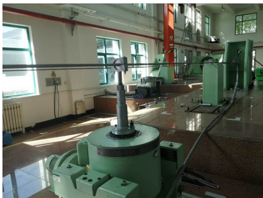
Fig. 5 Vibration exciter for simulating aeolian vibration.
