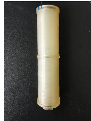
Fig. 4 Very-low-frequency interferometric FOH sensor head.
