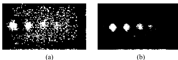
Fig. 15 Results of images processing by subtracting the gray reversal and denoising: (a) result of image before the gray reversal subtracting image after the gray reversal, and (b) denoise.
