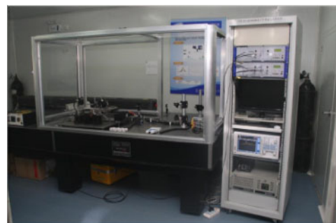
Fig. 7 Fabrication system of phase-shift grating using the phase mask: (a) structure diagram and (b) picture.
