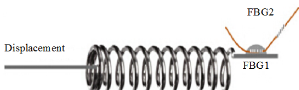
Fig. 5 Schematic of the sensing head of the long-range displacement sensor.
