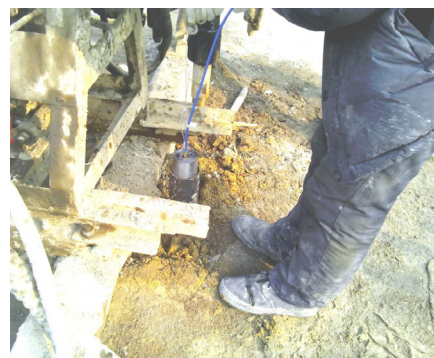
Fig. 9 Field installation of micro-seismic sensor.
