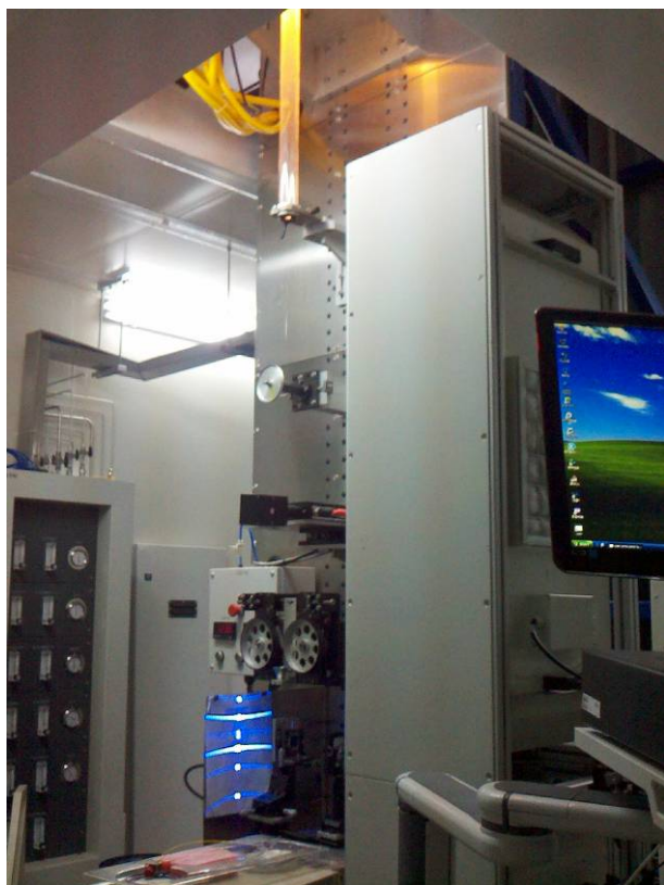
Fig. 1 Production-type draw-tower grating system.
