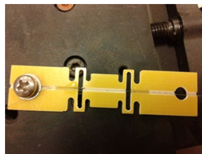
(b) FBG strain sensor packaged with FR-4
