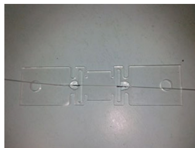
(a) FBG strain sensor packaged with silica
