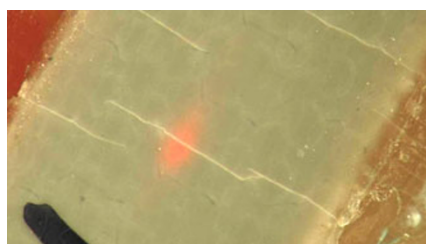
Fig. 13 Micro-crackings in Redux® packaging.
