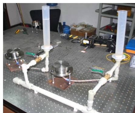
Fig. 40 Photo of FBG settlement sensors.
